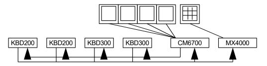
In this configuration all of the keyboards will provide limited control of the multiplexers Main monitor display only. These commands are activated by pressing the shift key and selecting the desired multiplexer function. The MX4000 will listen to all commands but only respond to those associated with multiplexer functions. The MX4000 will not send any information back to the keyboards or the CM6700.
